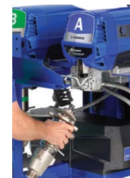
3. Remove hose and slide pump out
