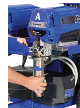
2. Open door and remove pump
